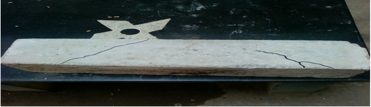
Figure 5(a): Shear failure pattern of R.C.C beam
