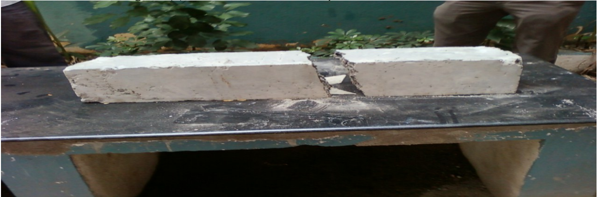
Figure 5(c): Failure pattern of P.C.C beam
